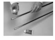
Replace the outer slide, moving it back and forth to spread the lubricant evenly.
